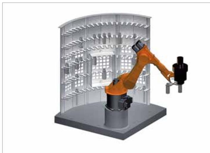
Vertical tool change directly into machine spindle
